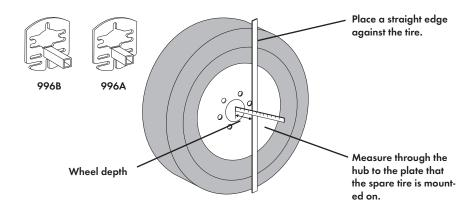
If the wheel depth (distance from spare tire mounting plate to outside of tire) is between 5" and 7-3/4" you must use Base Plate 996B. If the wheel depth is between 2-1/2" and 5-1/4", use Base Plate 996A. Measure through the hub to the plate that the spare tire is mounted on.
