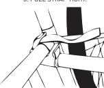
4. USE 70" STRAP (NOT INCLUDED) TO PULL ALL BICYCLES TOGETHER AROUND BOTTOM BRACKETS. STRAP SHOULD ALSO SECURE WHEELS.
