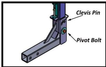
When you raise the arms of the bike rack to a 90 degree angle with the upright and then insert the attached Clevis pin into the hole, secure it with the snap pin. (Not shown)
