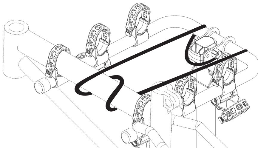
**Wrap strap around the last bicycle frame and the hitch rack arms (see illustration). We recommend using extra shock cord or rope on the bicycles to prevent the wheels from turning and to prevent the frames from swaying into each other. Do not allow the bicycle tires to rest close to the exhaust pipe to prevent them from melting. Check the bicycle(s) and hitch rack at regular intervals during use, more frequently on bumpy roads, and immediately if the bicycle(s) shift position.**
