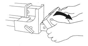
1. To store roll plate to vertical position, slide towards vehicle and lock.
