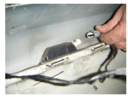
8. The first photo shows the bumper cover removed, exposing the aluminum bumper beam. Using a flat blade screwdriver remove the (7) wiring harness clips from the bumper beam.
