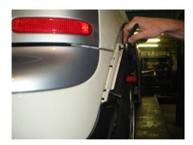
6. Using a phillips screwdriver, remove fastener 4 from the bottom of the bumper cover.
