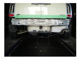
11. Secure hitch using (4) 8mm bolts and (4) 8mm nuts removed in Step (9). Torque all 8mm hardware to 24 ft-lbs.
