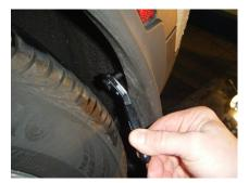
3. Using phillips screwdriver, remove fastener 2 from the bottom of the bumper near the rear wheel well. The second photo shows the optional mud flap removed.
